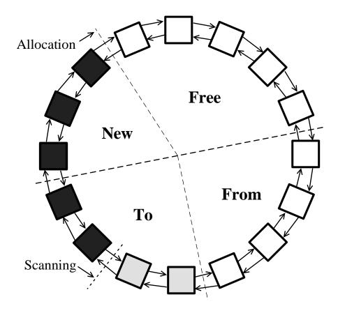
Fig. 8. Treadmill collector during collection.
